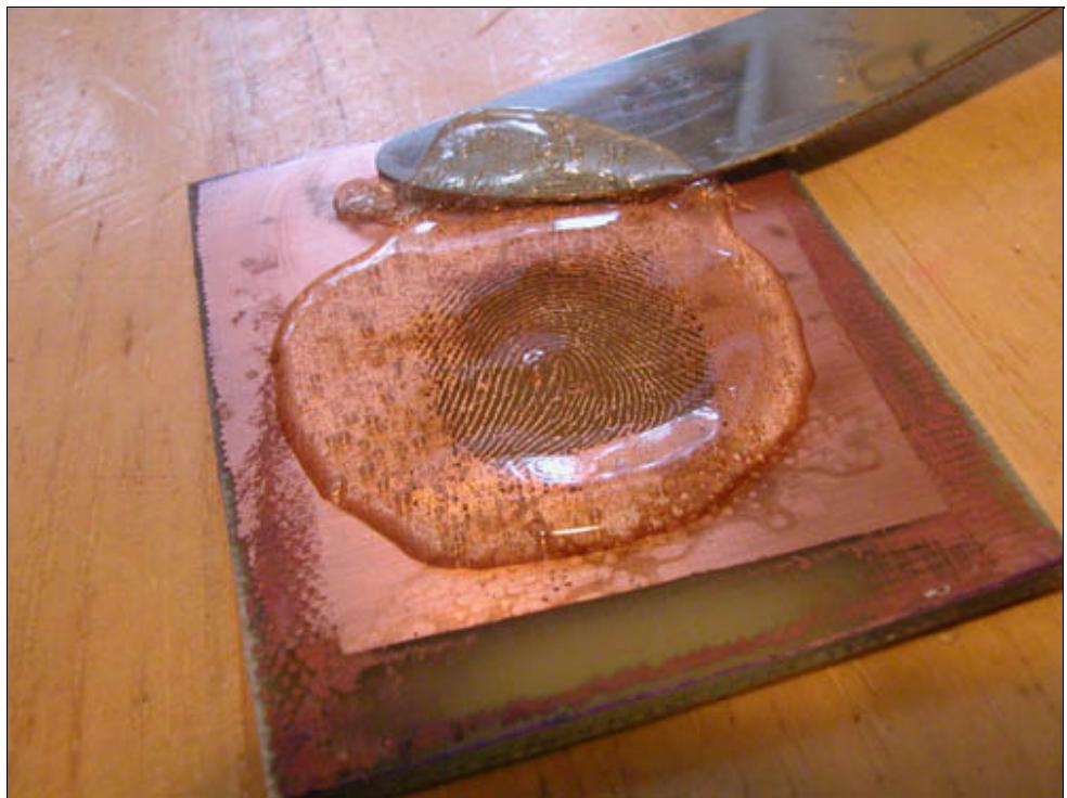
Fig3.6 - Gelatine spread on the board as a thin layer.
