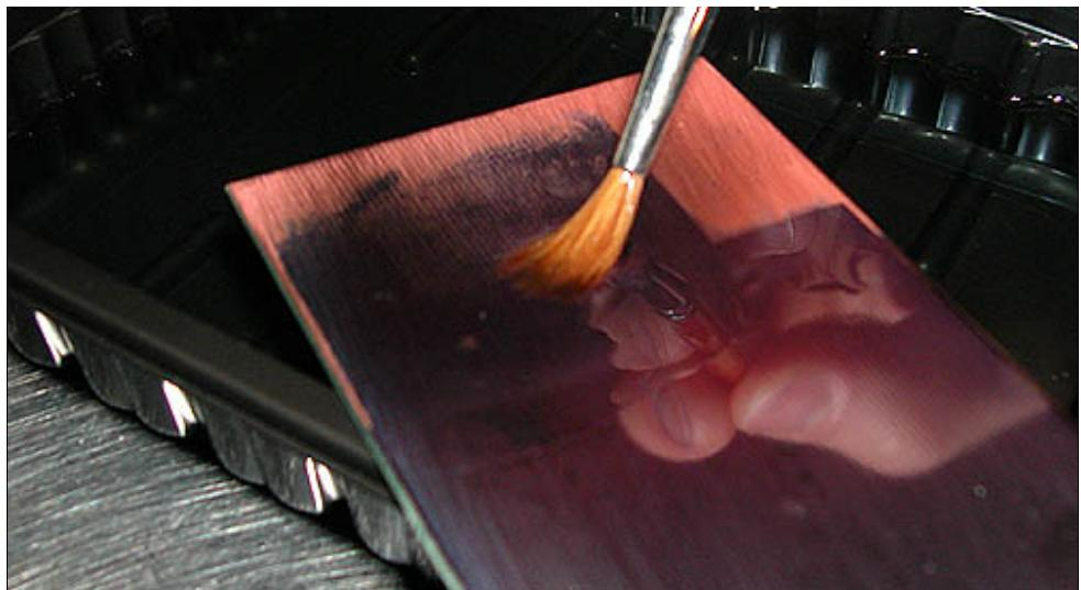
Fig3.3 - NaOH is used to wash off the lacquer in non-exposed areas.
