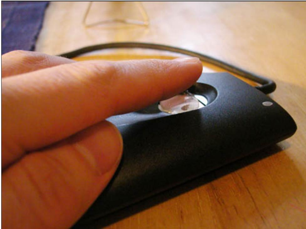
*Fig3.7 - Press the gelatine gently on the pad with the finger.*
