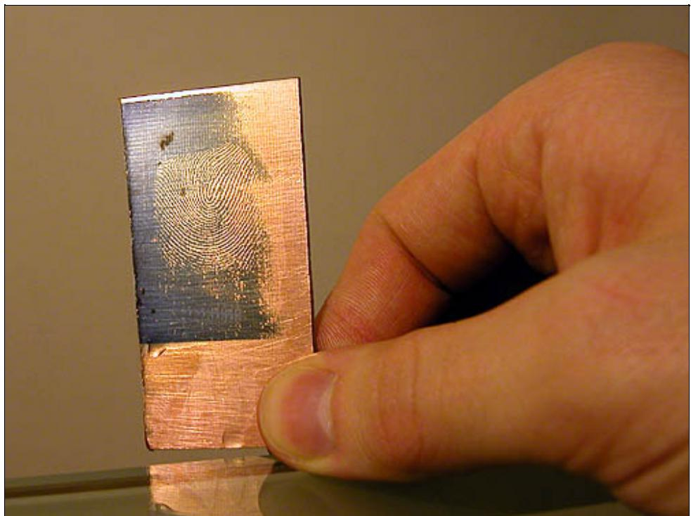
Fig3.4 - The board ready to be corroded.
